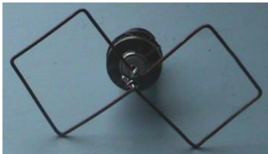
The "bowtie" and N-type connector assembly, before fitting to the ground plane.
