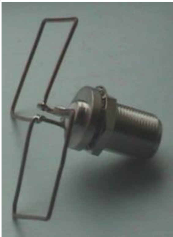
The "bowtie" and N-type connector assembly, before fitting to the ground plane.
